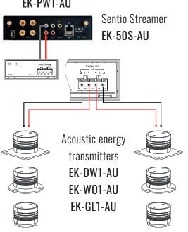
Connection 2-channel stereo on 4  $\Omega$ . Single transmitter applied power: 80 W
