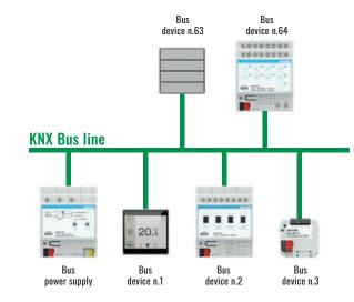
Next to a simple single-line configuration, a bus line can be subdivided into more segments, thus obtaining a star-shaped or a tree-shaped topology, or any combinations of the two.
