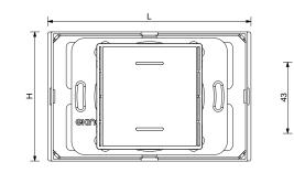
Mounting with frame: 122 x 77 (L x H) Mounting without frame ('NF): 120 x 80 (L x H)
