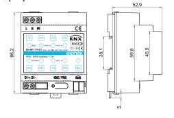
ETS application v.5 and 6 for configuring the KNX functions of the device. DCA App as special interface for configuring DALI segments.
