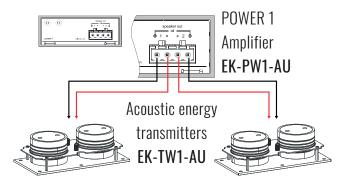
Connection 2-channel stereo on 4  $\Omega$ . Single transmitter applied power: 80 W
