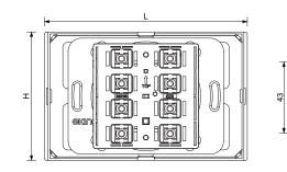
Mounting with frame: 122 x 77 (L x H) Mounting without frame ('NF): 120 x 80 (L x H)
