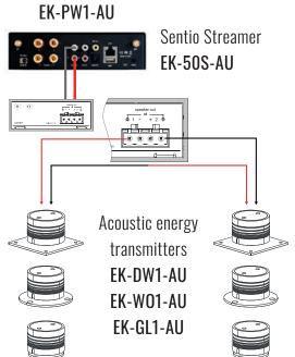
Series connection 1 mono channel on 8  $\Omega$ . Single transmitter applied power: 80 W
