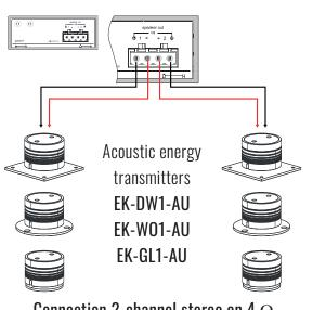
Connection 2-channel stereo on 4  $\Omega$ . Single transmitter applied power: 80 W
