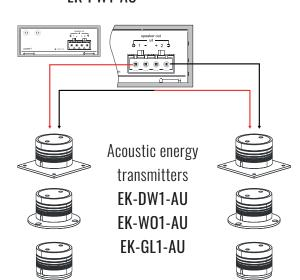
Series connection 1 mono channel on 8  $\Omega$ . Single transmitter applied power: 80 W
