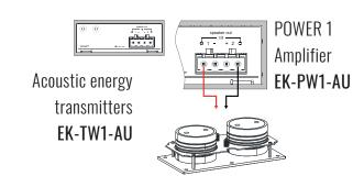
Connection 1 mono channel on 4  $\Omega$ . Single transmitter applied power: 200 W
