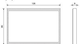
Rectangular frame of Flank version for finishing Ekinex® devices of FF and 71 series. Available in several colours and materials.
