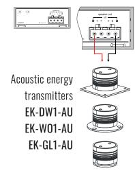
Connection 1 mono channel on 4  $\Omega$ . Single transmitter applied power: 200 W
