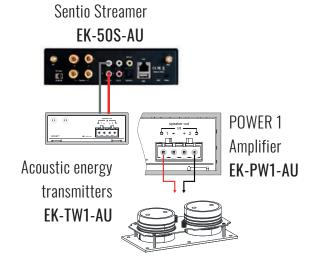
Connection 1 mono channel on 4  $\Omega$ . Single transmitter applied power: 200 W
