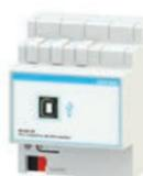
**CODESYS PLC with KNX interface**
