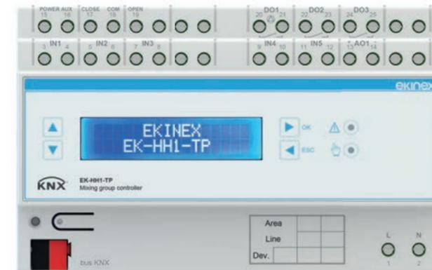
The display allows the operating parameters to be monitored; some control parameters can also be modified with respect to the initial configuration carried out with ETS. The switchover of the system conduction mode (heating / cooling) can be done from the bus, from a digital input (configured for this purpose) or manually from the front keyboard. Alarms from anti-condensation probes can be managed.
